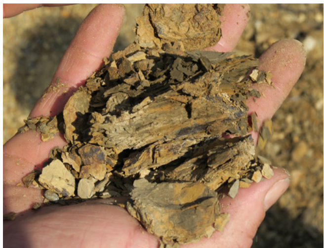
Compacted marl known locally as ponca
